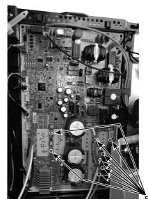
Screws of the inverter P.C. board
