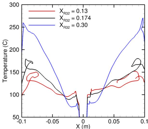
**Figure 7:** Temperature profiles along the  $x$  direction of different contours of constant R-32 concentration: 0.13 (which corresponds to lower flammability limit at ambient conditions) in red, 0.174 (stoichiometric) in black, and 0.3 (which corresponds to upper flammability limit at ambient conditions) in blue. Data were extracted from Figure 6c and correspond to averaged values over 0.5 s.
