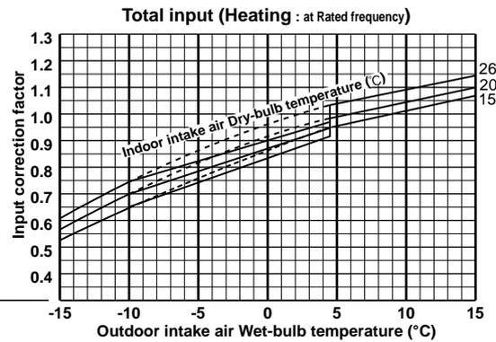
**NOTE:** The above broken lines are for the heating operation without any frost and defrost operation.
