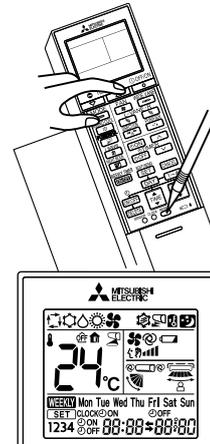
Press STOP/OPERATE (OFF/ON) button of the remote controller (the set temperature is displayed) with the remote controller headed towards the indoor unit. ※1
